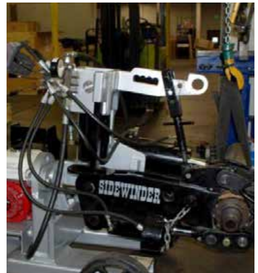
27. Use valve handle 1 to extend the wrench breakout cylinder and open the hammer joint. If the hammer slips in the jaws use both valve handles 2 and 3 to increase the hold pressure. Increase this by about 250-500 psi.
