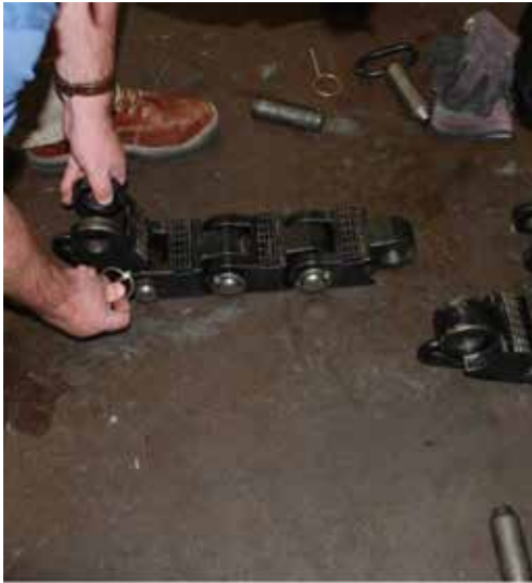
4. Remove the cotter pin from the link with handle on both the fixed arm and moveable arm.
