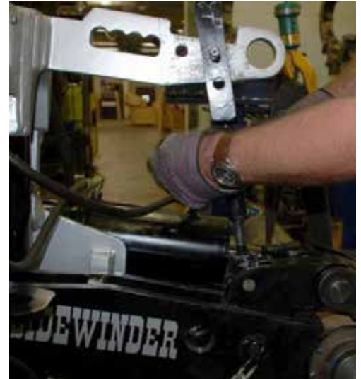
24. Rotate the adjusting screw to align the jaw of the moveable arm with the work piece.
