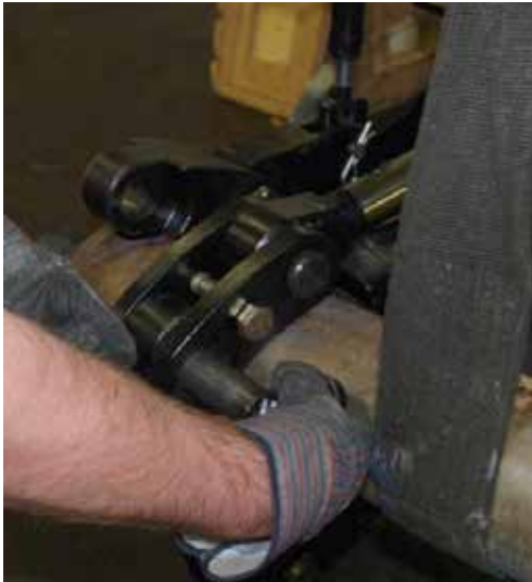
16. Lift the link with handle around the hammer and secure it with the pin with handle.
