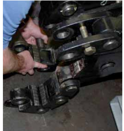
6. Secure the link with handle onto the end of the remaining links on both the fixed arm and moveable arm.
