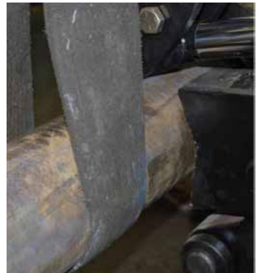
15. Use appropriate lifting equipment and position the hammer so that the wear sleeve is centralized with the V of the fixed arm.
