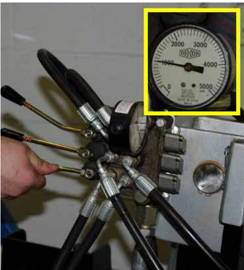
25. Use valve handle 3 to close the wrench chain cylinder on the moveable arm, stopping when the pressure gauge reads 1000 psi.
