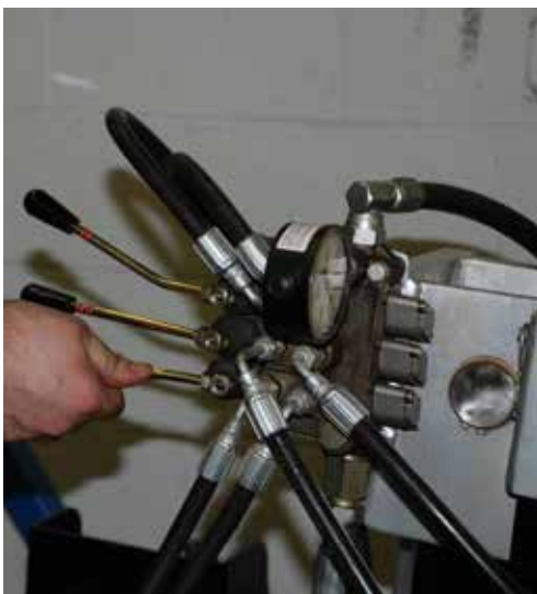
19. Use valve handle 3 to fully extend the wrench chain cylinder on the moveable arm.
