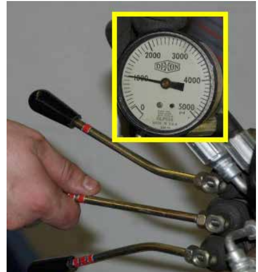
18. Set the throttle to half and pull valve 2 to close the fixed jaw cylinder. Stop when the gauge reaches 1000 psi. Valve handle 2 will not be used again until the hammer is open unless slippage occurs at the fixed arm jaw.
