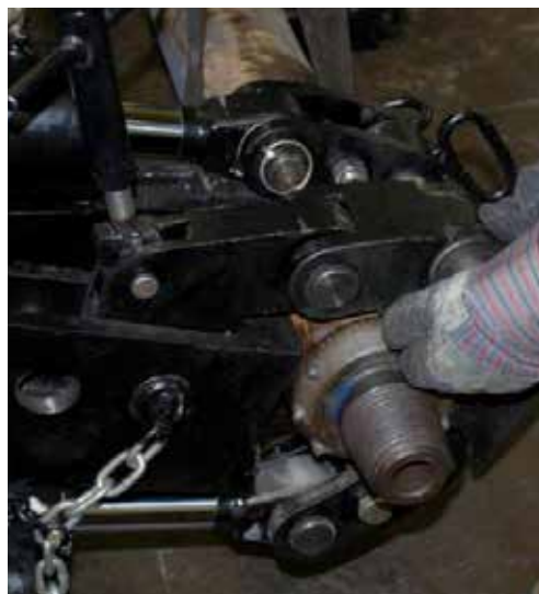
20. With the cylinder fully extended, lift the chain using the link with handle and secure it in place with the pin with handle.
