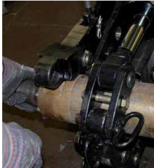
17. Align the hammer so that the chuck or backhead is in line with the moveable arm jaw, and the joint is outside the grip of the jaw.
