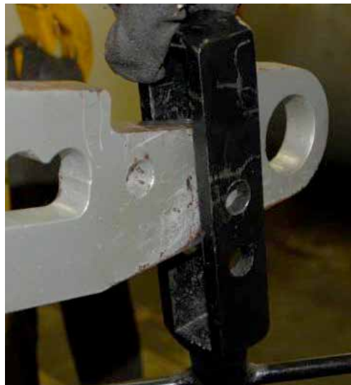
26. Remove the pin from the adjusting screw so that it is loose.
